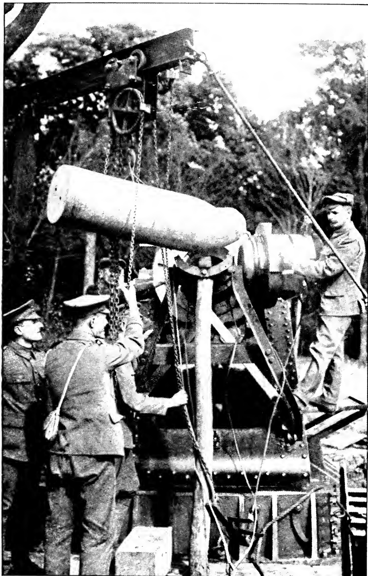
BRITISH SOLDIERS HOISTING A SHELL INTO A 15-IN. HOWITZER
